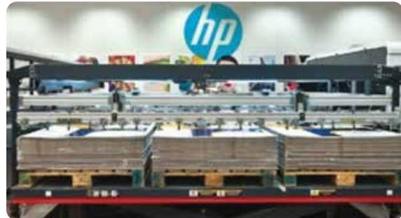
Barberan's Jetmaster BIJB-1260 corrugated press is 1,260mm wide, with a lead-edge feeder that leaves 5mm between sheets, with delivery onto a conveyor that can lead to a stacker. It prints at up to 55m per minute at 360dpi resolution and three grey levels. "So far the 1260 is our widest printer, but we have projects to go wider, up to 1,980mm," says van Ijzerloo.
