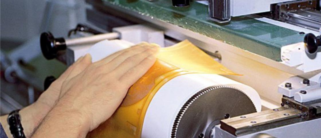
durometer (hardness) of the plate along with the surface tension of the face. Hardness and surface tension both affect the ink releasing characteristics of the plate. When the plate is out of spec, then the press operator is left to try to compensate through non standard ink and impression settings. It is at this point that the plate is ready to be trimmed to its finished dimensions. The trimming of the photopolymer plate can be performed either by the platemaker of the plate mouter.
