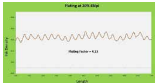
Graph of a printed scan with a Fluting Factor of 4.13
